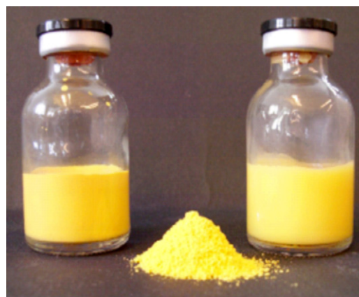
Fig. 3. Aqueous coenzyme Q10 nanosuspensions, size 219 nm (left), lyophilized nanocrystal power (middle) and redispersed lyophilized powder in Milli-Q water (right). The size after redispersion is only slightly higher, 263 nm (photon correlation spectroscopy data) (by courtesy after Mauludin, 2008).
